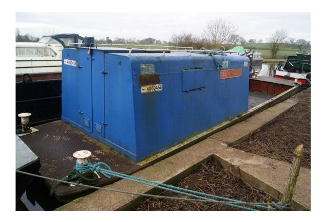
36ft unpowered welfare/work boat. Cabin at rear with bench seating, worktop with sink and space for a multifuel stove. Toilet compartment and tool store. Large open hold. The hull of this boat has been overplated.
